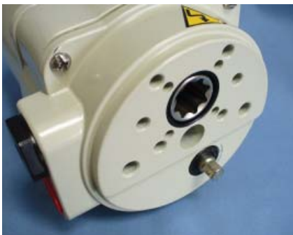
ISO F03/05 Mounting Detail, 8mm socket override and 8 point 14mm female drive on P1 Series actuators.
